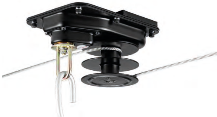
Ceiling mountable 2270 kg / 11 m With shared reel, which makes reeling possible from opposite directions with two wires. Equipped with brake which keeps the load in place. The brake and gears are protected from dust and rain. Can be used for lifting.
