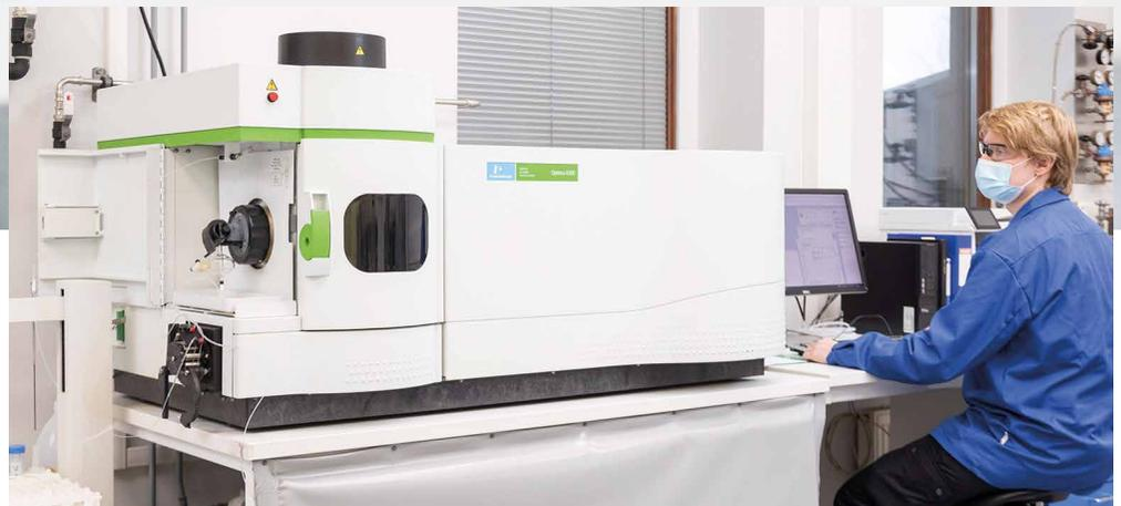
The workhorse of the laboratory is **ICP-OES**, which is used to determine the metal composition of materials. The results can be used to determine the prices of precious metal materials.
