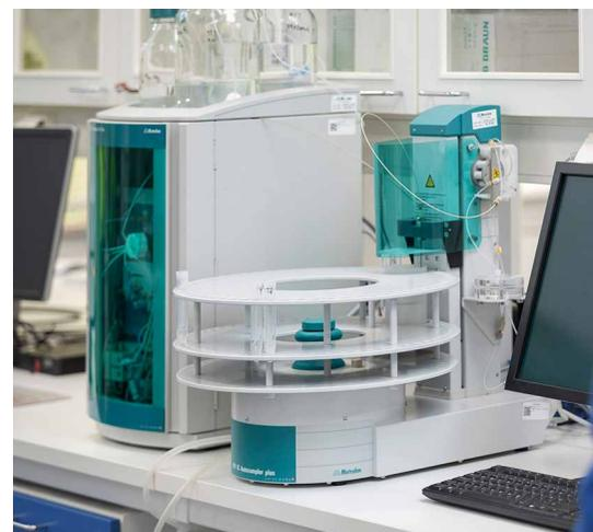
**Ion Chromatography (IC)** is used to analyse chlorine and sulphur in solid recovered fuels.
