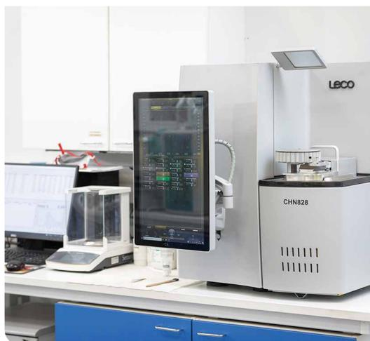
A **LECO CHN828** elemental analyser is the laboratory's latest acquisition and is used to analyse carbon, hydrogen and nitrogen levels in solid recovered fuels.
