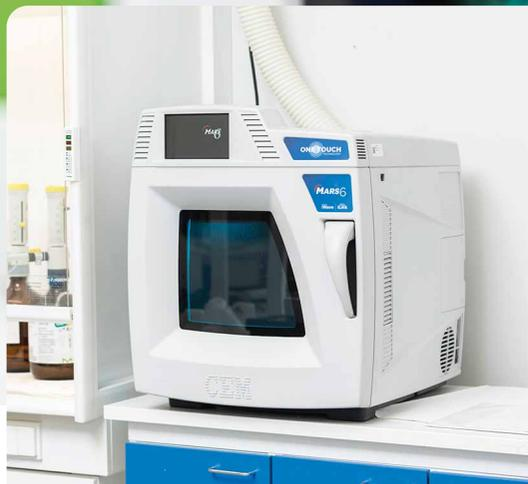
**Microwave digestion** is used to pretreat samples before they are analysed.
