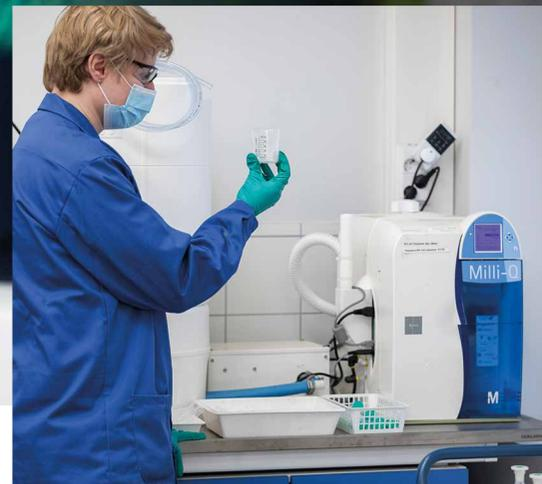
**Milli-Q** equipment ensures that the water used in the analyses is ultrapure.
