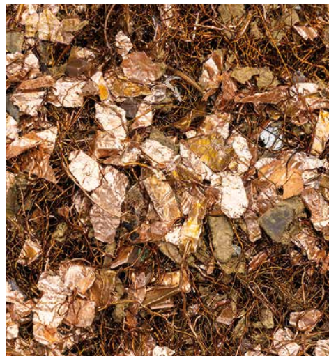
Copper granulate made from transformers.
