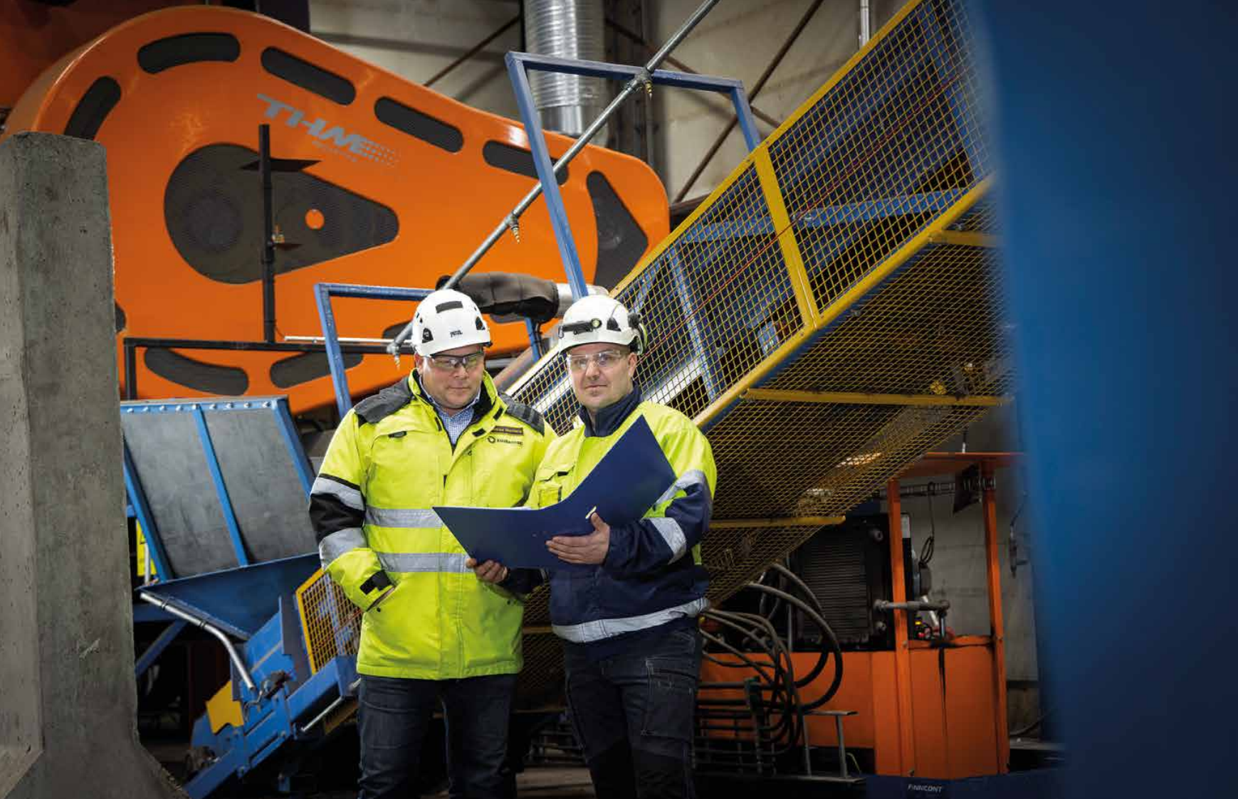
The progress of the investment project has been closely followed by Tuomas Mantere , Production Director, and Marko Serkosalmi , Project Manager for Machinery and Equipment. The new 38-tonne shredder can be seen in the background. The shredder is used to pre-process the copper- and aluminium-containing materials delivered to the copper centre.
