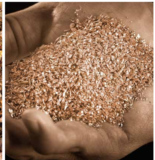
Copper granulate made from cables.
