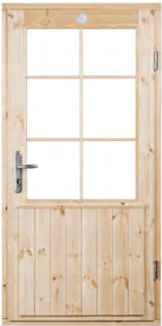
DOOR TYPE C10 , 897 × 1820 mm DOOR TYPE C24 , 897 × 1960 mm Glass: Float 4 mm or Thermo-security 4/6/4 mm
