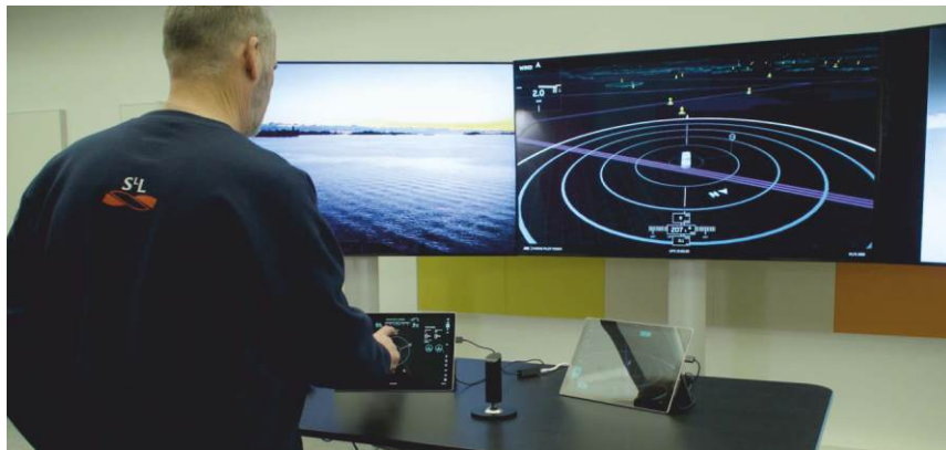
Remote control was tested on the Suomenlinna II ferry in 2018. ABB technology was used. The picture shows a view of the remote control centre. Photo: ©ABB
